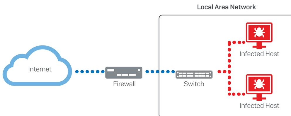
A best practice is to segment the LAN into smaller subnets using zones or VLANs and then connecting these together through the firewall to enable the application of anti-malware and IPS protection between segments that can effectively identify and block threats attempting to move laterally on the network.
